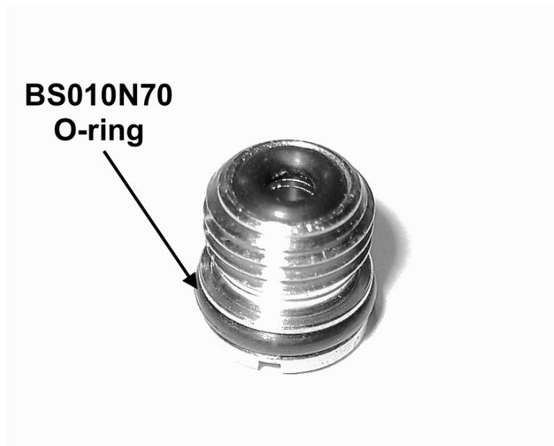
When this O-ring is damaged, diluent gas will leak into the loop. Also, removing it has a high risk of damaging it in the process. Therefore ALWAYS replace this O-ring when servicing the ADV.
