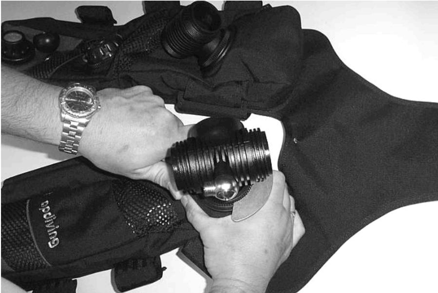
Screw the ADV on to the retainer base and tighten it up using RBTOOL 6.
