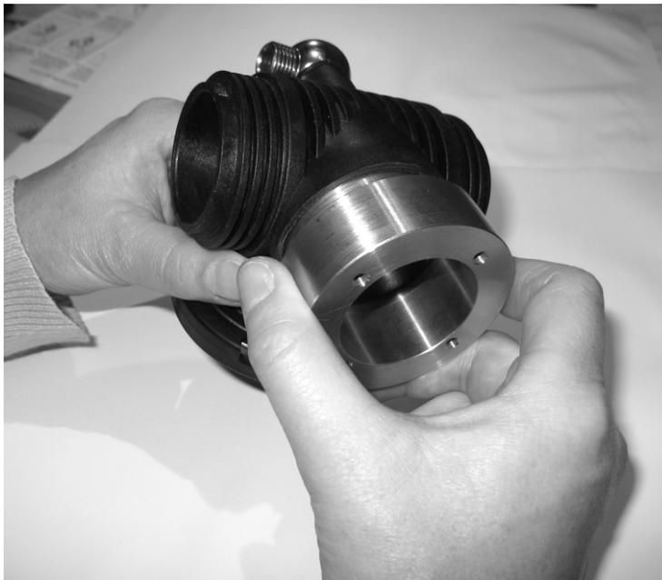
Screw clockwise, using special tool RB TOOL 8 or a pair of pliers with thin tips that fit correctly. Make sure that the 4 pins from the special tool are properly locked into the 4 small holes in the locking ring to avoid damaging the ring.
