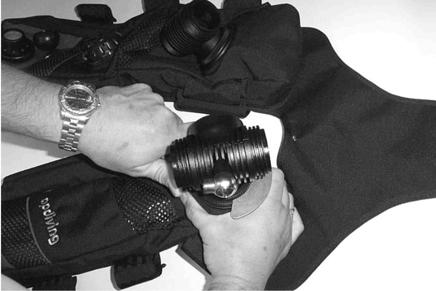
Use RBTOOL 6 to hold the Top, while your other hand grips the Retainer Base through the counterlung outer bag.
