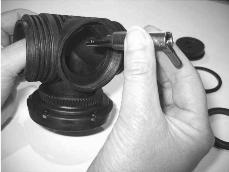
The BS014 O-ring on the outside of the banjo seals on the outer face of the ADV. Make sure you push it through carefully, without levering.
