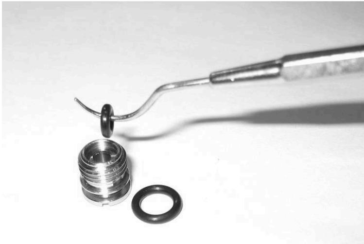
This small O-ring has a very special role. It acts as the valve seat for the tilt-axle which acts as an up-stream valve. Together with the tilt-axle they act as the core valve assembly of the ADV. Damage to this O-ring will lead to a leaking ADV. Therefore ALWAYS replace it when servicing the ADV.
